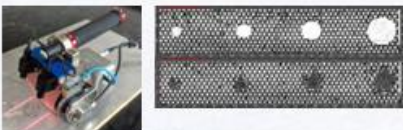
Inspection of Aviation Aluminum Honeycomb Panel
